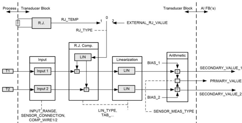
Figure 5.3 Transducer block structure
