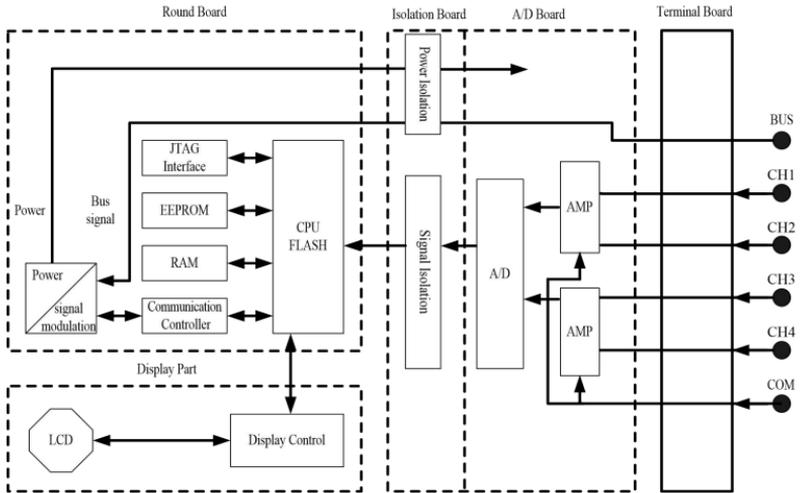
Figure 3.1 Schematic diagram of NCS-TT105 temperature transmitter
