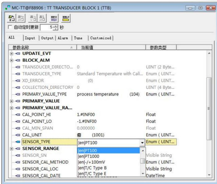
Figure 4.3 Sensor type configuration
