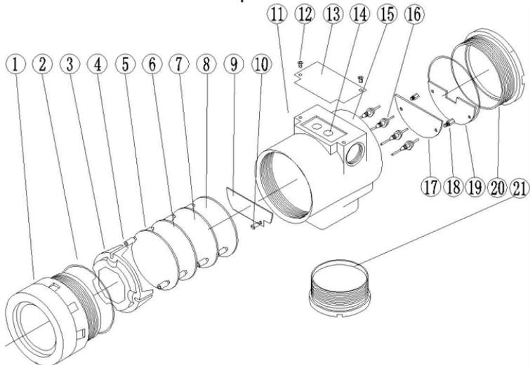
Figure 3.3 Structure of NCS-TT105 temperature transmitter
