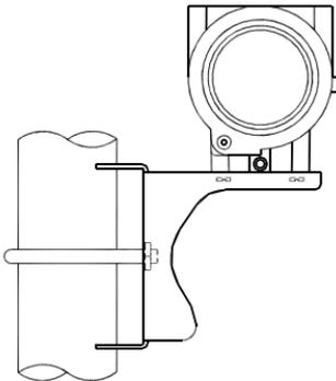
Figure 2.3 The installation of pipe mounting angle bracket-1
