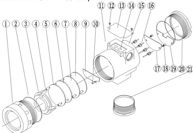
Figure 3.3 Structure of NCS-TT105 temperature transmitter
