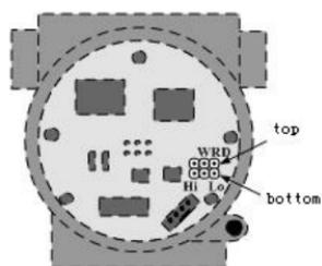
Figure 6.5 HART smart transmitter hardware jumper
