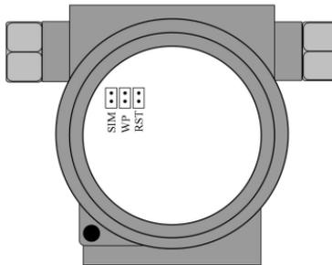
Figure 4.7 NCS-TT105 temperature transmitter hardware jumpers
