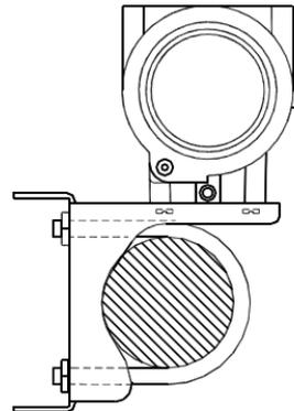
Figure 2.4 The installation of pipe mounting angle bracket-2
