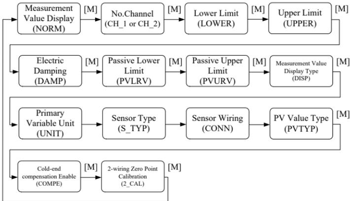
Figure 7.4 Adjusting Function and LCD Display
