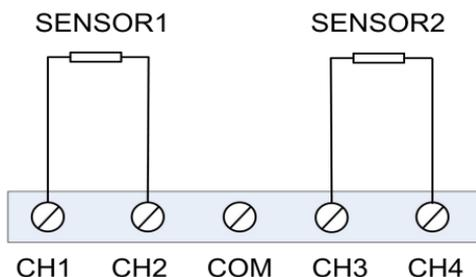
Figure 2.7 Wiring of NCS-TT105 temperature transmitter(2-wire)
