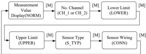
Figure 7.2 Adjusting function and LCD display
