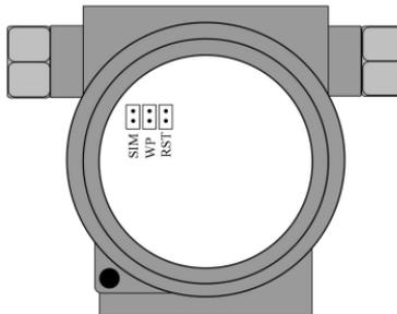
Figure 4.7 NCS-TT105 temperature transmitter hardware jumpers
