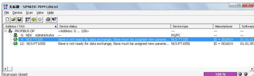
Figure 5.9 Scan DP bus and List PA device
