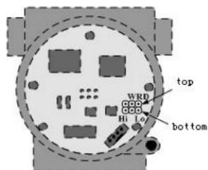
Figure 6.5 HART smart transmitter hardware jumper
