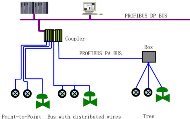
Figure 5.1 PRFIBUS PA network topology
