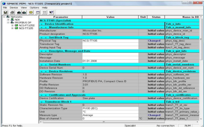
Figure 5.11 Device Management with PDM software
