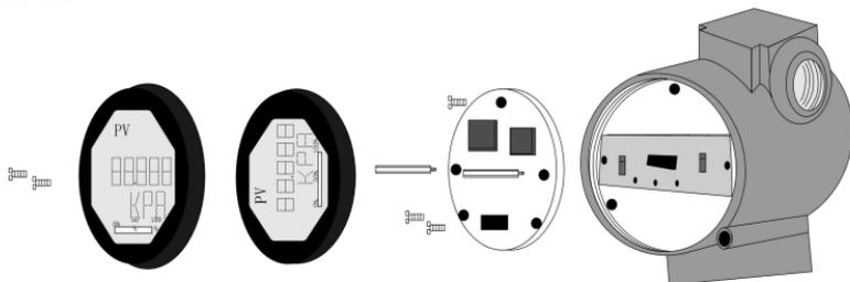
Figure 3.4 Assembly structure of the transmitter
