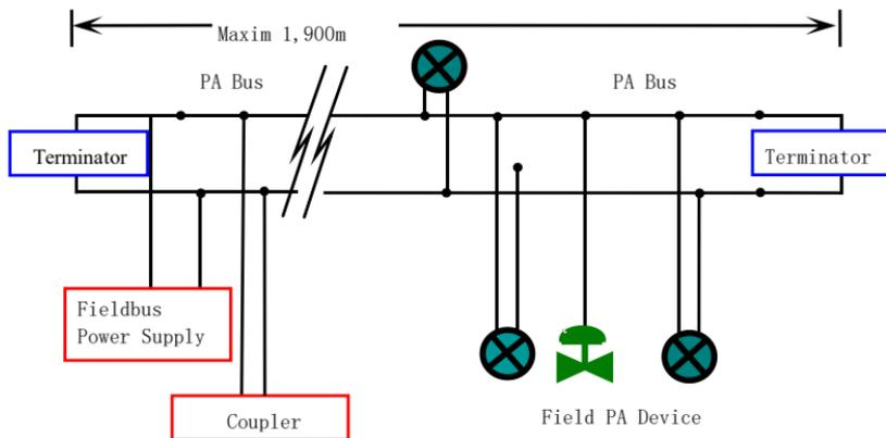
Figure 5.2 PRFIBUS PA bus connection
