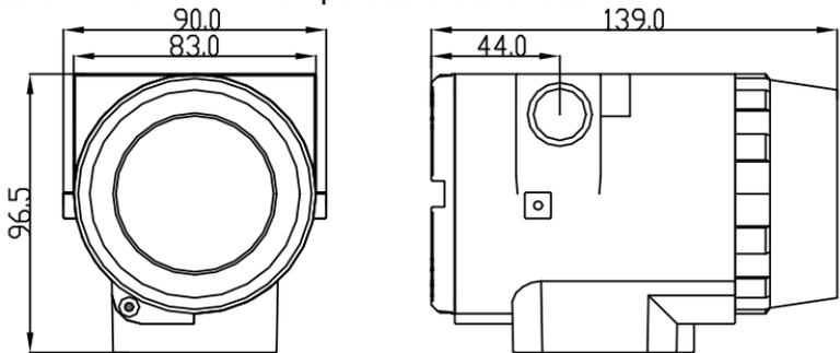
Figure 3.2 Size of NCS-TT105 temperature transmitter (unit: mm)
